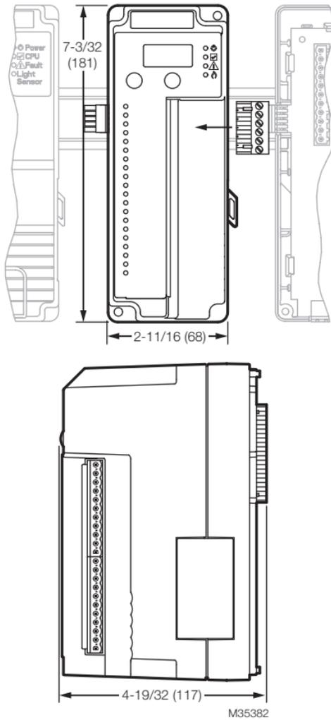
Fig. 1. Dimensions in in. (mm).
